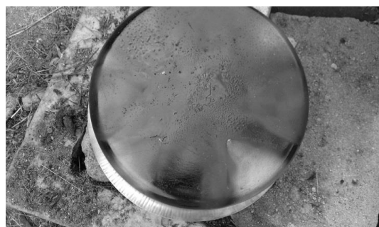
Figure 6. Typical soot with tar on pot bottom after cooking on natural draft TLUD stove with pellets.
