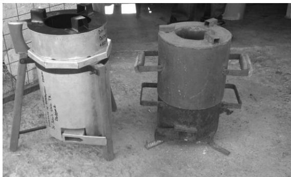
Figure 2. Troika (left) and Jiko Bomba TLUD stoves. Primary air vent can be seen at bottom of both.
