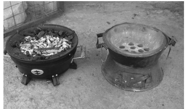
Figure 5. Charcoal stoves. Improved stove, left (Ecofit), traditional stove, right. Ecofit diameter is 31 cm.
